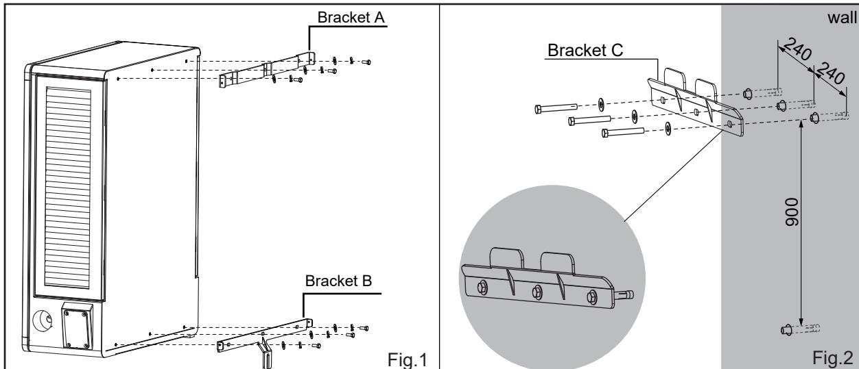
3. Install support C using the removed bolts and gaskets. The locking torque is 55N·m.
