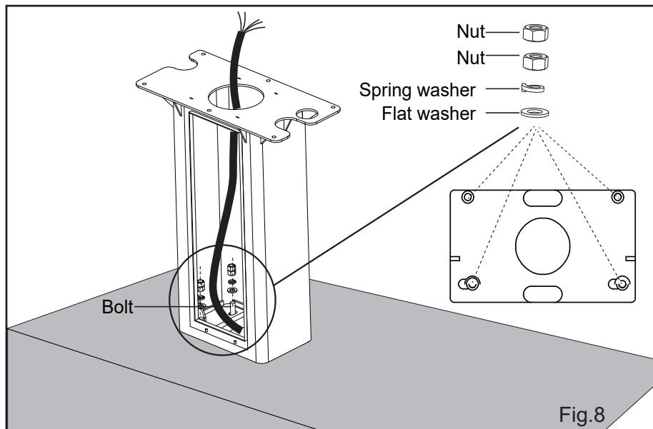
4. Install the unit on the base of the machine with 6 M8\* bolts according to Fig.9, and tighten the bolts in place and install and lock the rear panels.
