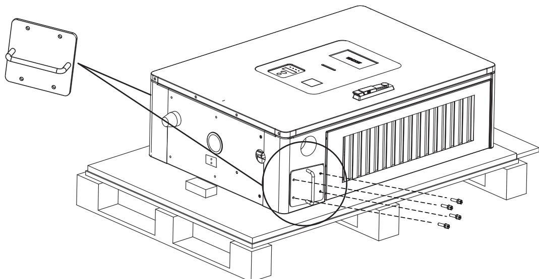
Take out the handle fittings, and fix the handle to the shell with 8 M6\*30 bolts according to the figure below, which is convenient for the handling and installation of the shell; After the installation is complete, remove it to facilitate subsequent installation of the gun mounting base. Secure the side without the gun mounting base of the single-gun machine to the mounting hole of the gun mounting base using four M6\*30 bolts.
