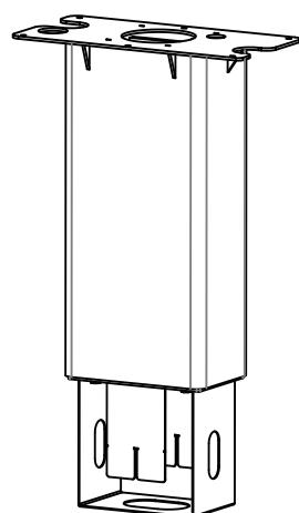
Stand fixing bracket and pedestal assembly\*\*
