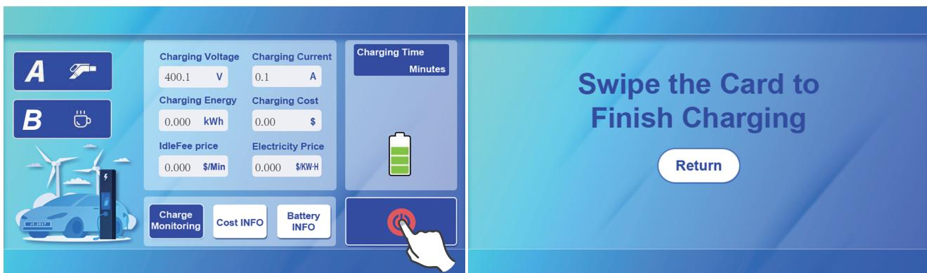
This interface can view charging fee information: Charging energy, Cost, Charging time, Current, Idle Fee Cost, Idle time.
